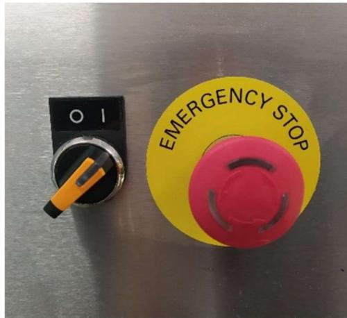
Rotate the power switch to position 1
