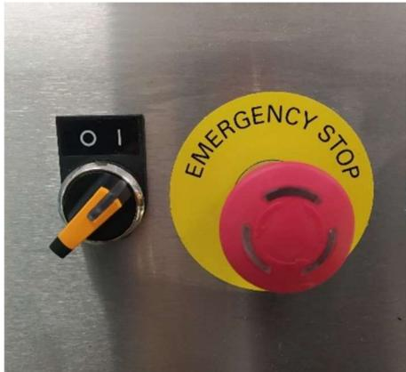
Rotate the electrical switch to position 0
