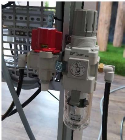
Rotate the main switch to position sup
