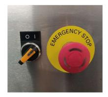
Rotate the power switch to position 1
