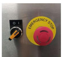
Rotate the eletrical switch to position 0
