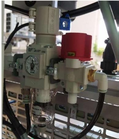
Rotate the main switch to position sup
