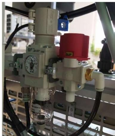
Rotate the station air switch to position sup
