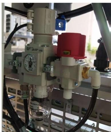
Rotate the main switch to position sup
