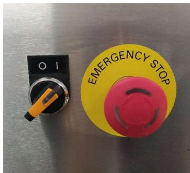
Rotate the power switch to position 1
