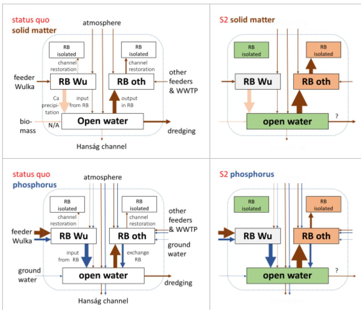
Figure 41. Alteration of matter flows for sediment (upper) and phosphorus (lower) in scenario S2.
