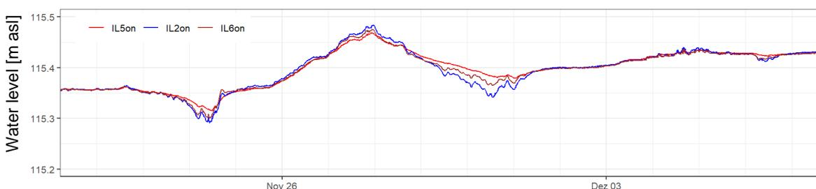
**Figure 11. Course of the water level at three monitoring stations in the reed belt of Illmitz between 22 Nov and 7 Dec 2018. Station IL5on lies in a large, open brown-water area with >14 ha; a rise of water level of 10 cm corresponds to a water inflow of >14 000 m<sup>3</sup>.**
