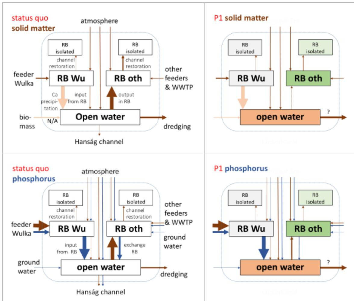
Figure 30. Alteration of matter flows for sediment (upper) and phosphorus (lower) in scenario P1.
