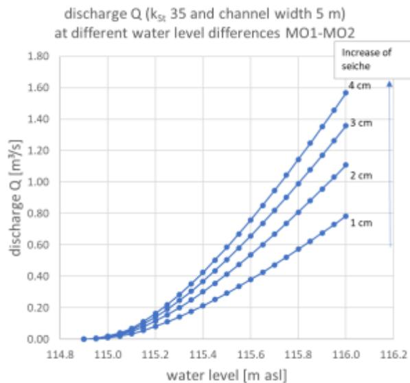
**Figure 29.** Relation between water level and discharge through a channel near Mörbisch assuming varying water level differences (MO1 lake edge, MO2 reed belt) resulting from a seiche wave (model after Manning-Strickler).
