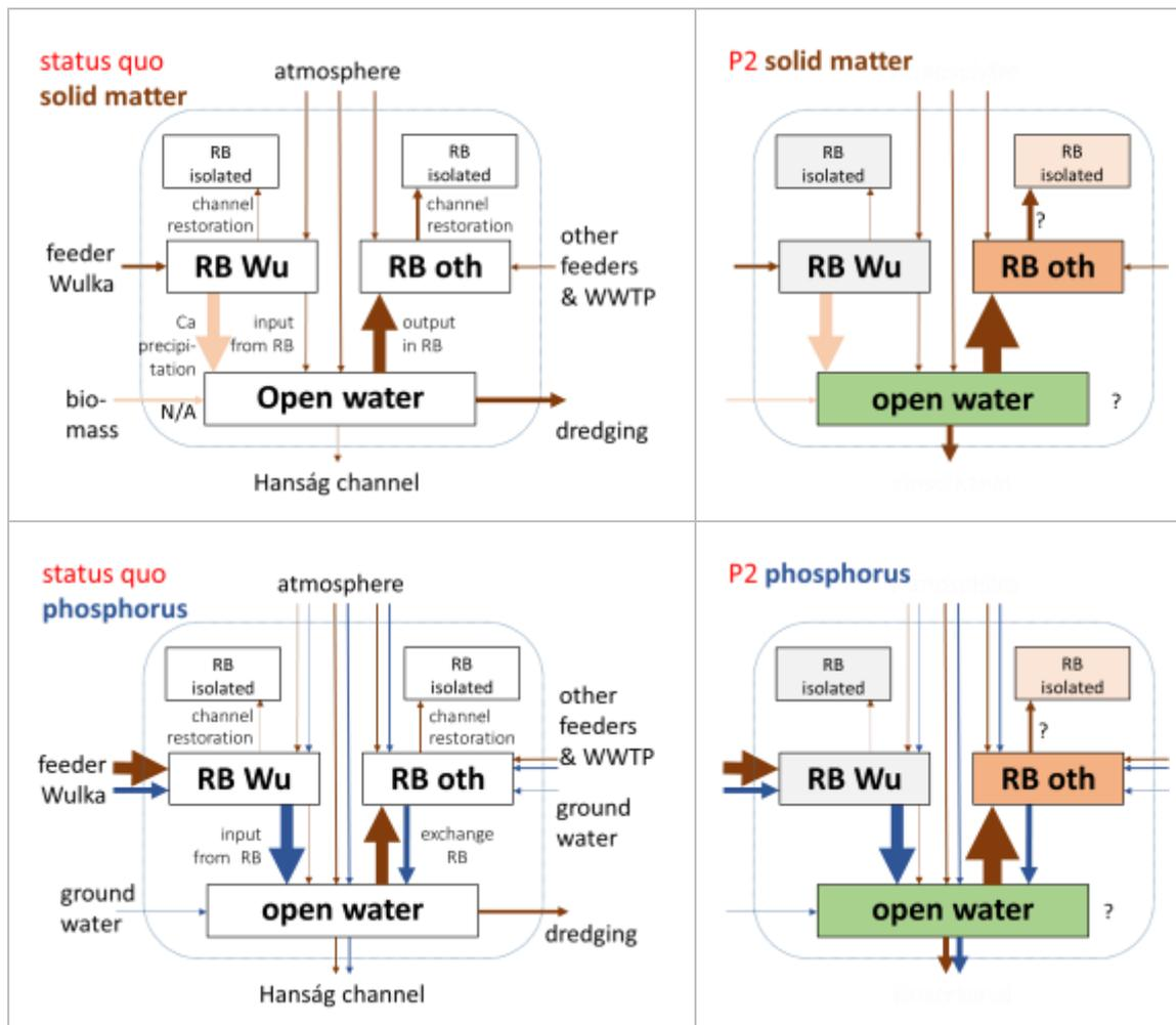
Figure 32. Alteration of matter flows for sediment (upper) and phosphorus (lower) in scenario P2.
