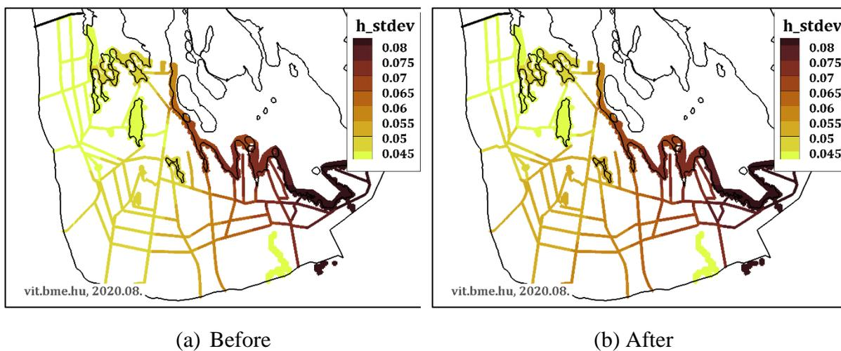
**Figure 38.** Standard deviation of wind induced water level fluctuations in the channels (a) before the reconstruction and (b) at present, modelled for low water level (115.30 m asl), in [m].
