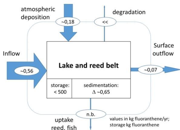
Figure 19. Estimation of a substance balance of the Lake Neusiedl / Fertő for fluoranthene (long term water balance combined with substance concentrations from 2017–2019).
