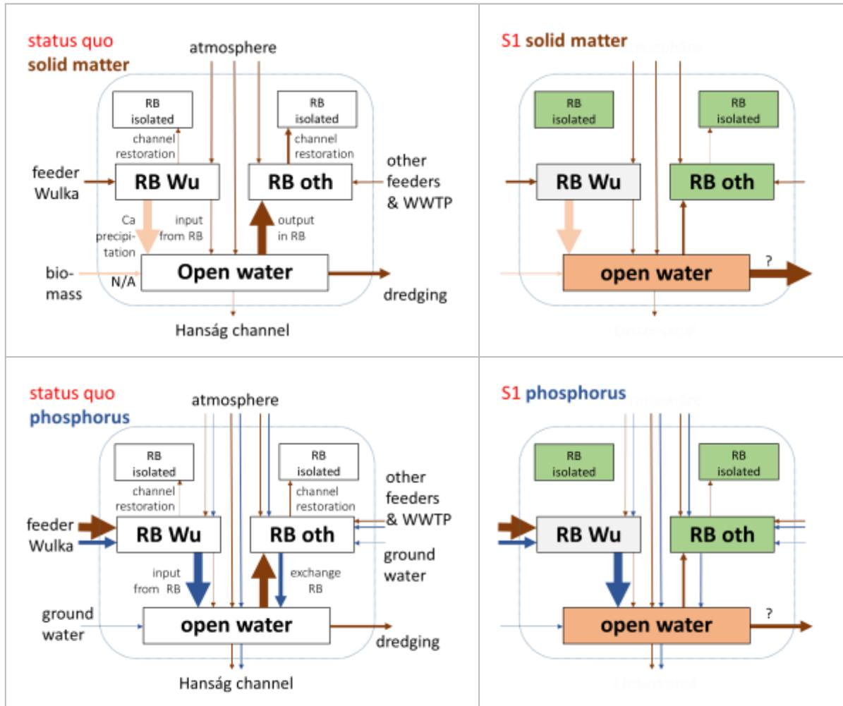
Figure 35. Alteration of matter flows for sediment (upper) and phosphorus (lower) in scenario S1.
