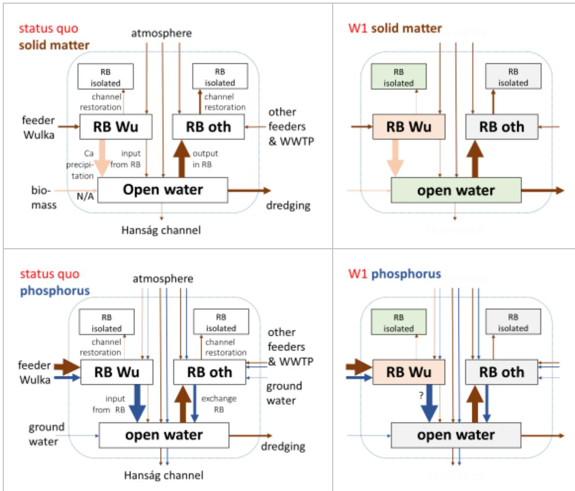
Figure 33. Alteration of matter flows for sediment (upper) and phosphorus (lower) in scenario W1.
