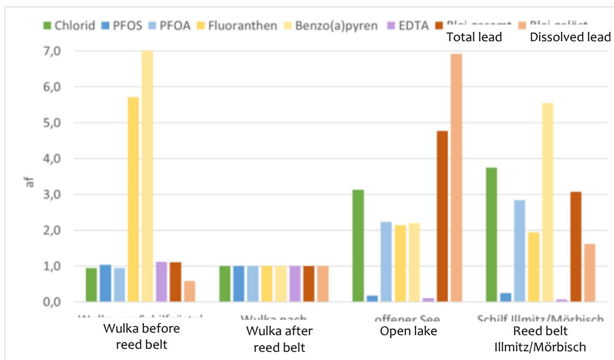
**Figure 17. Enrichment or decrease factor ( $af = C_n/C_0$ ) for selected substances.  $C_n$  means concentrations in each water phase and  $C_0$  was chosen the concentrations in the inflow from the Wulka reed belt to the open lake.**
