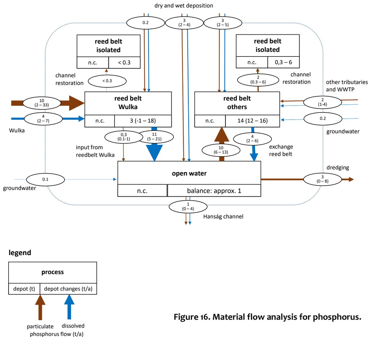
Figure 16. Material flow analysis for phosphorus.
