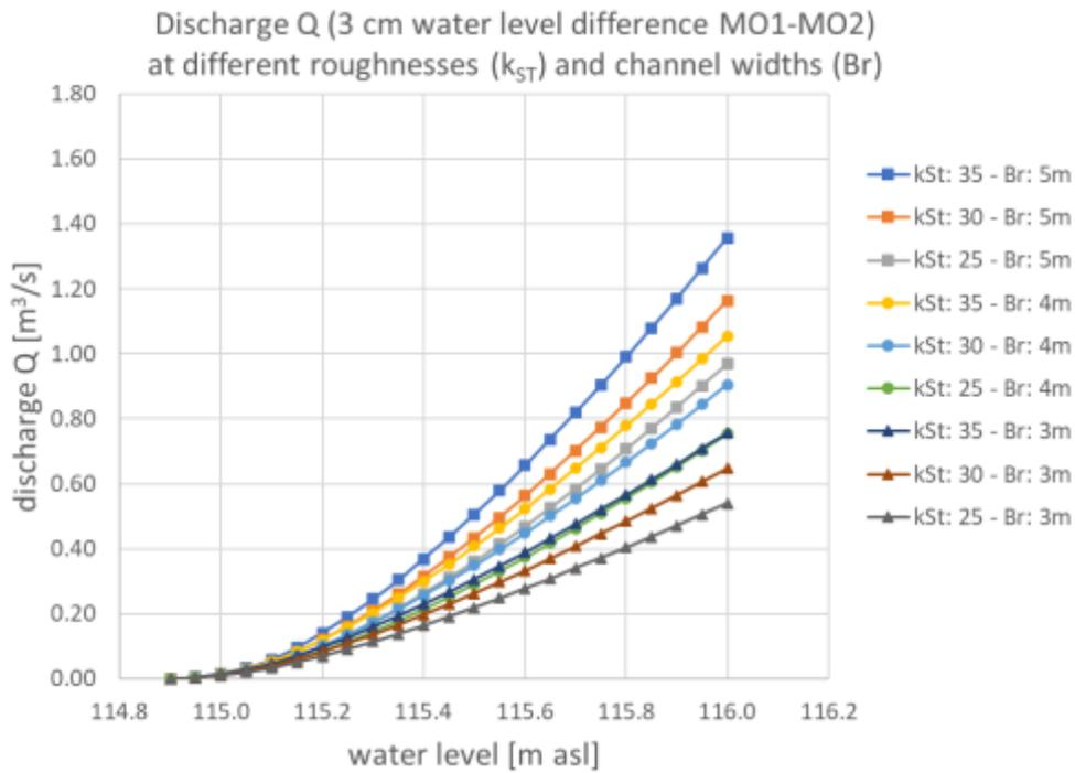
Figure 36. Relation between water level and discharge through a channel near Mörbisch assuming varying channel width, using the Manning-Strickler model (MO1 lake edge, MO2 reed belt).
