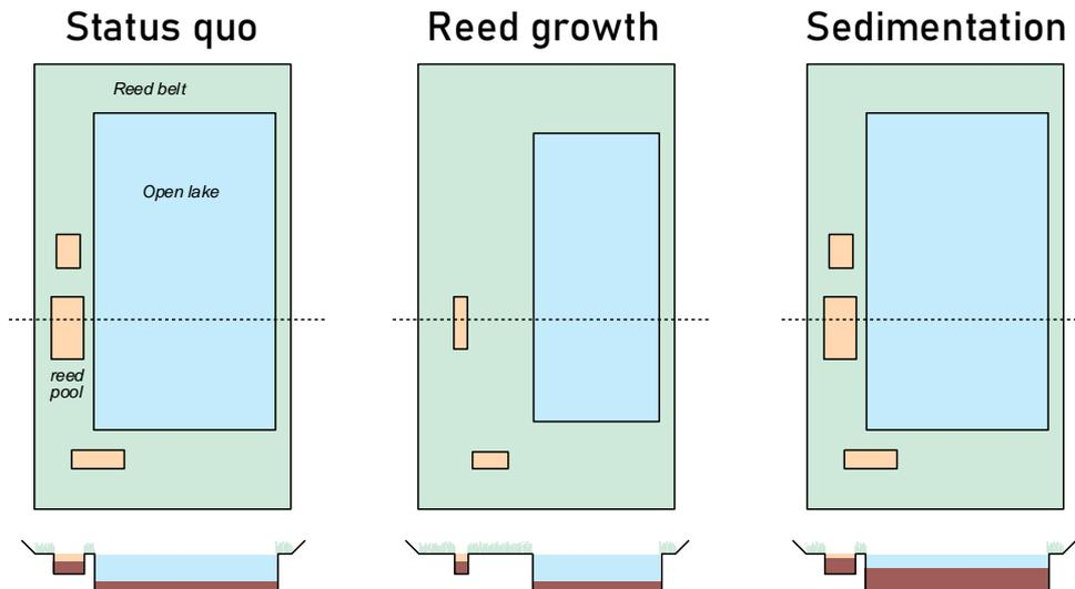
Figure 23. Schematic drawing of “Verlandung” in the sense of an increase of reed stands (middle) and of sedimentation (right).
