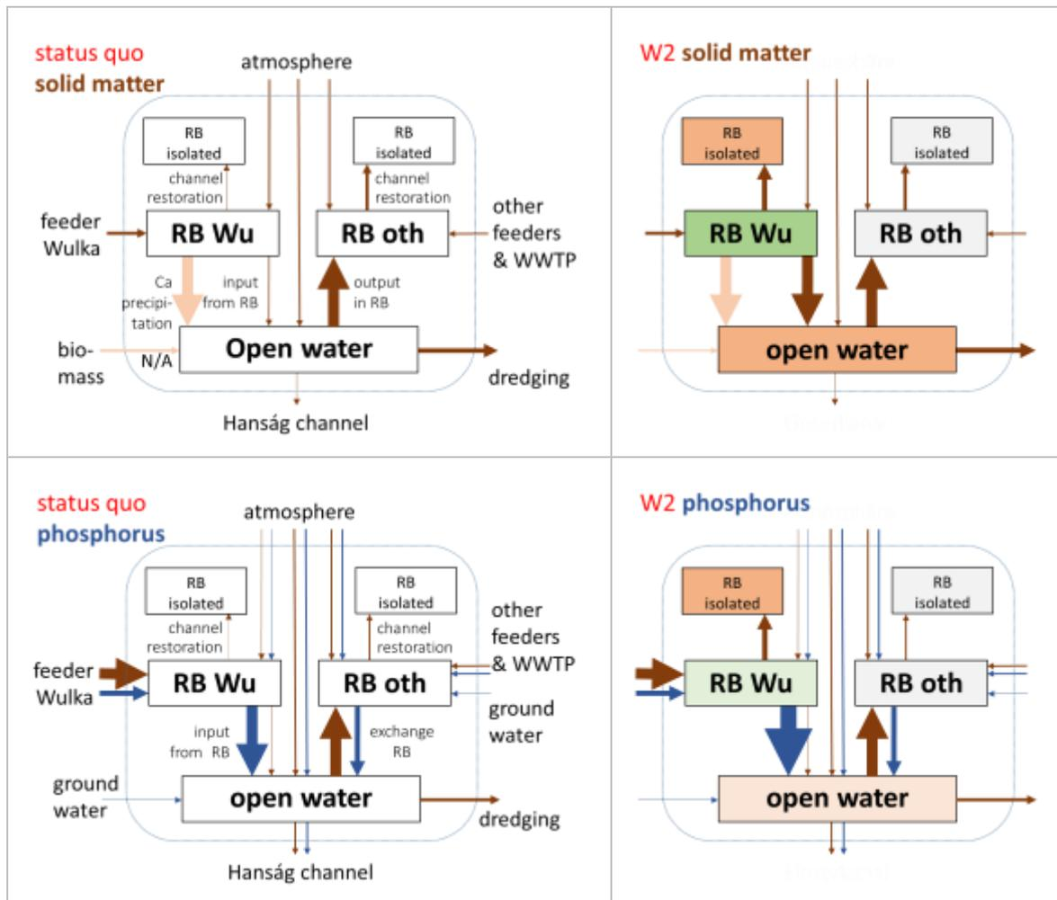
Figure 34. Alteration of matter flows for sediment (upper) and phosphorus (lower) in scenario W2.
