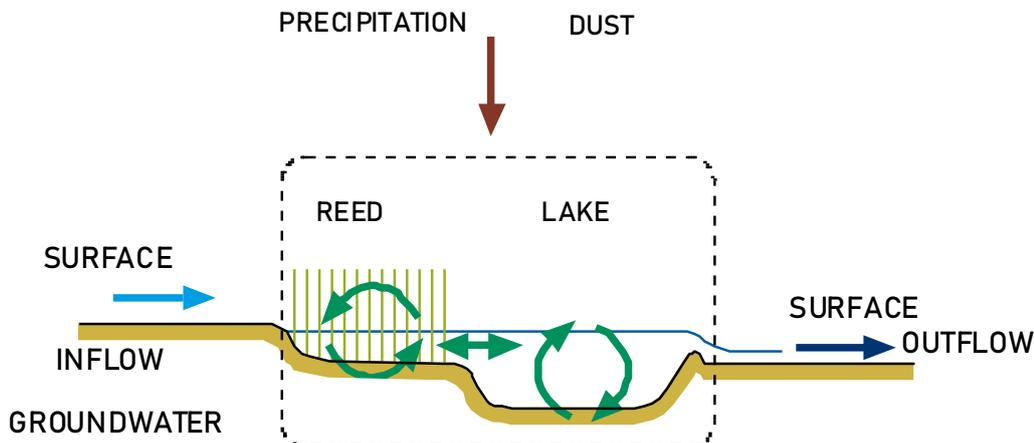
**Figure 1. Scheme of inputs, outputs, and internal processes in Lake Neusiedl / Fertő. Source: Stalzer & Spatzierer (1987) (modified).**
