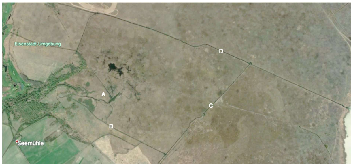
Figure 2. Channels at the mouth of the river Wulka into Lake Neusiedl. Most recent channel dredging occurred between A and B. Channel B – C is the preferred pathway of the river at low discharge. At high discharge, a significant part of the river flows also through channel D.
